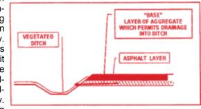
cold weather, freezing and thawing of water trapped in the base under the pavement causes rapid deterioration of the pavement. An open ditch of sufficient depth provides continuous drainage of the base.
