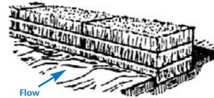
2. Place bales in trench with bindings around sides away from the ground. Leave no gaps between bales.
